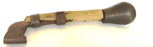
Antique turpentine hack blade or hook. It was used to cut the “V” shaped marks in the side of the tree as shown in the photo at top-left. The “V” shaped marks are permanent and are called a “cat face.” Source: https://www.worthpoint.com/worthopedia/antique-turpentine-hack-blade-tar-1784881577
