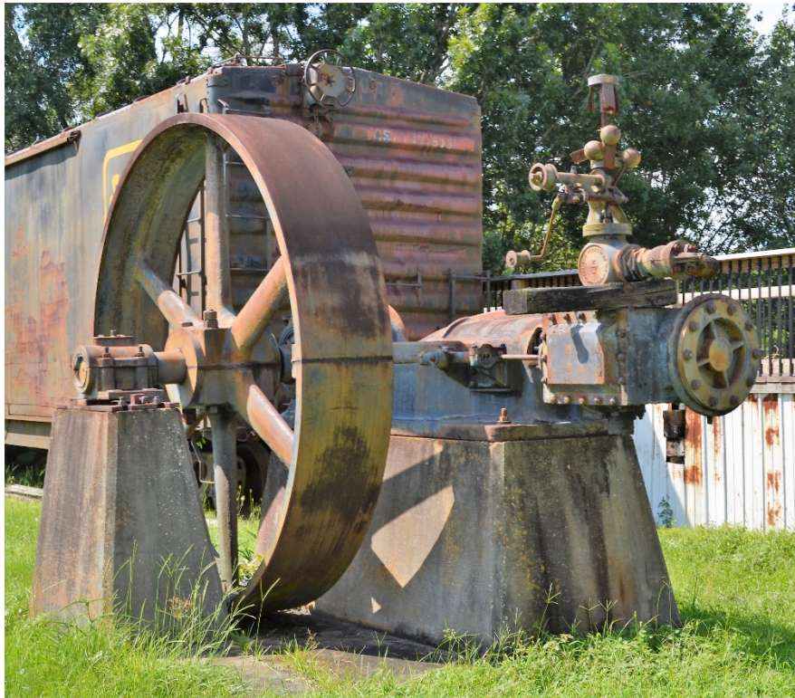
The steam engine pictured in the two photos above is on display at the L & N depot in Florala. It came from the Jaxkson veneer mill once located in Laurel Hill, Florida. The Florala Saw Mill Company and other saw mills in the area used steam engines of this type to power their machinery. Photos by Sam Carnley, 7/22/2021.
